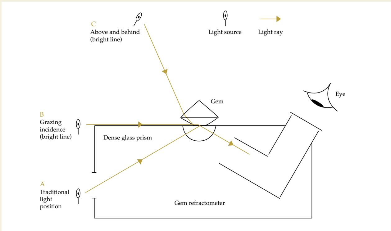
Figure 5: Diagram of a refractometer showing the positions a, b and c of a light source for traditional illumination, and for grazing incidence.
