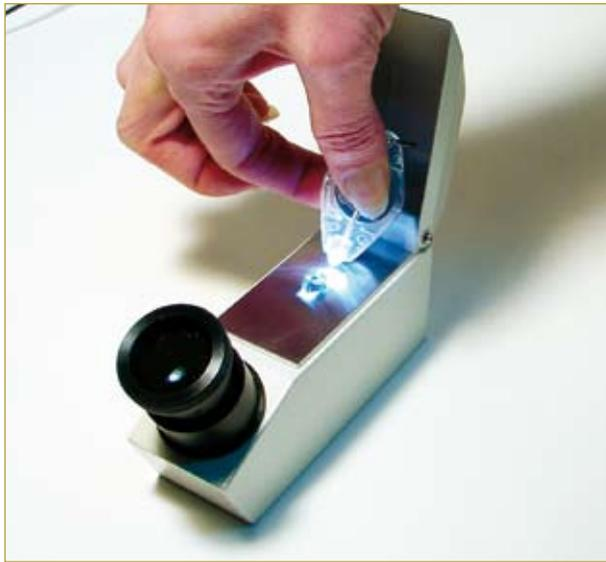
**Figure 2:** Modern style refractometer with small LED light directed at grazing incidence.
