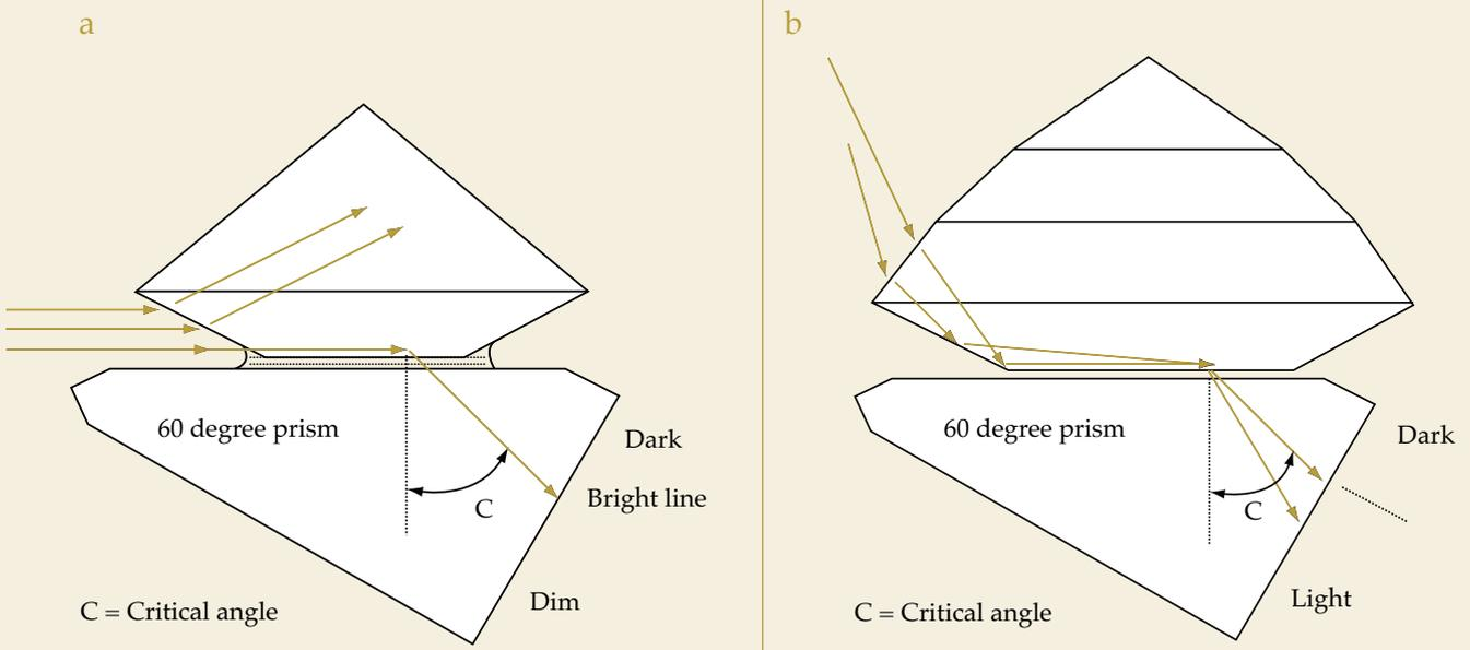
Figure 6: Sketch of the light paths in the prism of a gemmologist's refractometer when grazing incidence is used. In position (a) light is directed in the plane of the prism surface. In position (b), light is directed into a pavilion facet from above and behind.
