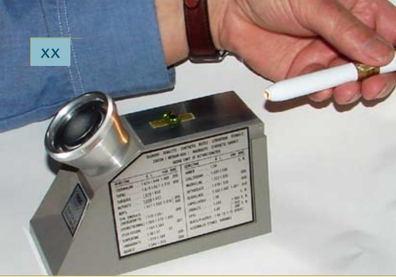
**Figure 1:** A critical angle refractometer with the light shield removed and illuminated for grazing incidence using a torch.
