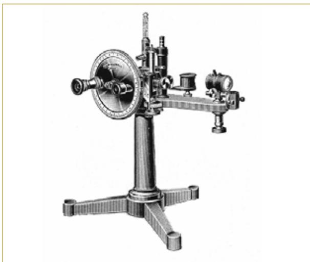
**Figure 3:** Pulfrich refractometer, catalog scan taken from Arthur H. Thomas Co. Laboratory Apparatus and Reagents. Philadelphia (1921).
